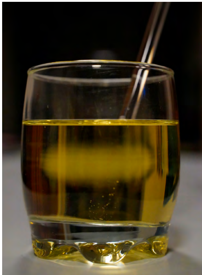
This borosilicate glass stirring rod is invisible in the oil. Credit: Elise Adams
